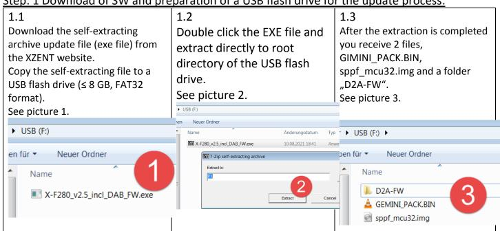
Attention: in some rare cases, the USB-flash-drive may not be detected by the XZENT device. If one step fails, please re-check and re-use a different brand/manufacturer USB flash drive item and/or change the memory size (<1 GB, 2 GB, 4 GB ...).
