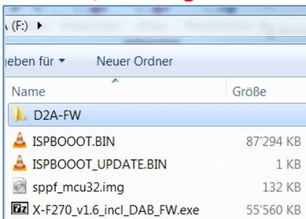
Double clicking the self-extracting file will produce 3 additional files and one folder – as shown in the picture above: ISPBOOT.BIN, ISPBOOT\_Update.BIN, sppf\_mcu32.img and the folder „D2A-FW“.
