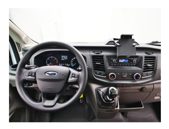
If the radio is replaced with a navigation system with a larger screen, the tablet holder can no longer be opened or will hit the edge of the screen when opened from above.
