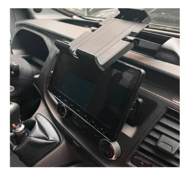
For this reason, we recommend removing the tablet holder where possible. Or replace it with the original FORD storage tray when installing the retrofit navigation solution.
